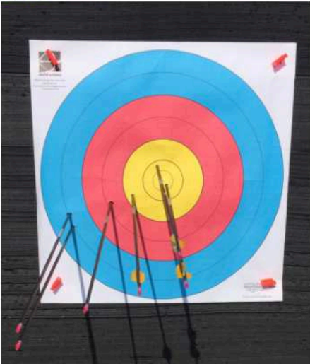
Figure 9a. Nock point too high, stiff arrow.
