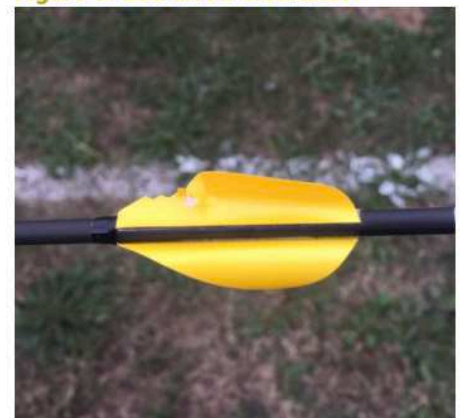
Figure 8. Bad arrow clearance.
